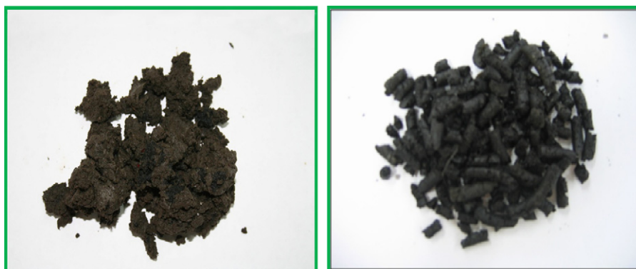
Fig. 3. Photography of before and after fry-drying chemical plant sludge.
